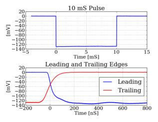
Figure 7: Pulse mode detected output RF.
