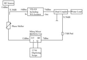
Figure 6: Measuring phase and amplitude ripple.
